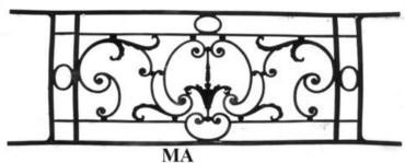
HT1: 511mm HT2: 337mm LG1: 1397mm LG2: 1105mm
