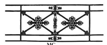
HT1: 530mm HT2:446mm HT3:358mm LG1: 1357mm
